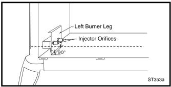
Fig. 64 Remove and replace injector orifices.
